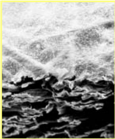
In this magnified view of an edge of Spider-Web® and the substrate media, we can see how dirt collects on the 'web' at the surface, instead of penetrating the media where it can clog media pores and restrict airflow. Donaldson Spider-Web® has very small pores (spaces between fibers) that allow air to pass through even as the media loads with particulate -- thus keeping ΔP low over the entire life of the filter.
