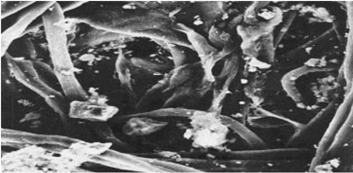
Figure 6 SEM micrograph of conventional filter material for engine air cleaner applications loaded with ISO fine test dust.
